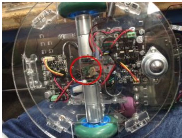
Figure 14: Location of the IMU on the drivetrain
